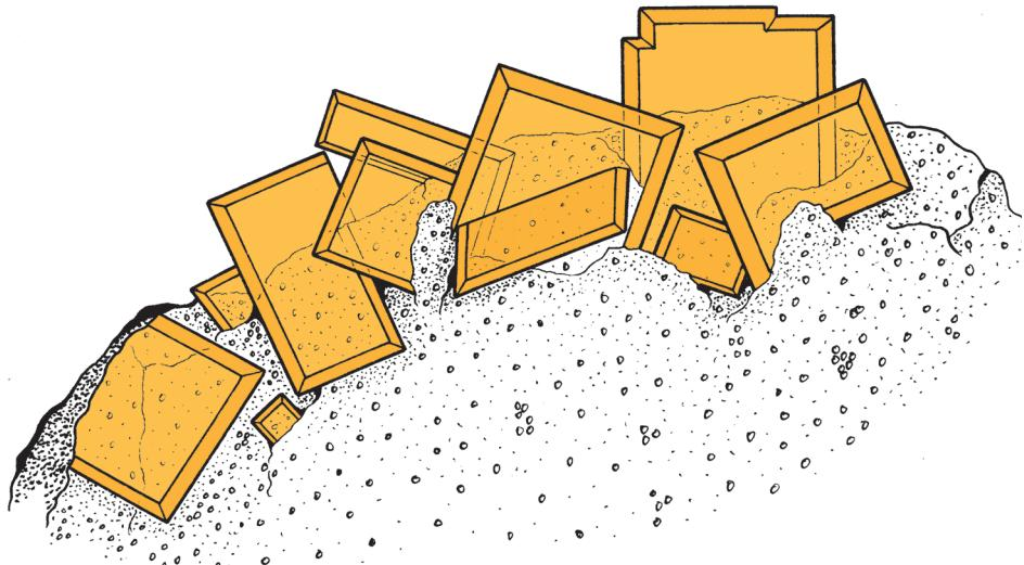
**Wulfenite, an ore of molybdenum**
